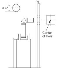
Figure 9 - Vent Opening Requirements
